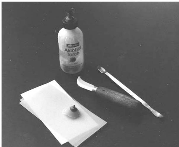
FIGURE 16 Tools used to alter wax shape include carving knife, spatula, and alcohol torch.
